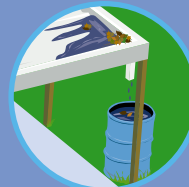
Flat roof without adequate drainage
